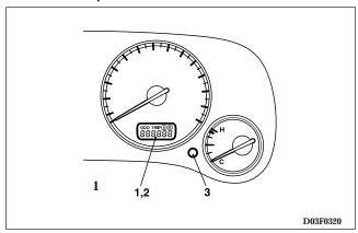
When the ignition switch is turned to the "ON" position, an "ODO" or "TRIP" indication is given.
